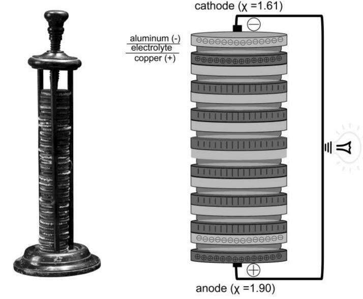
Electricity is *chemically* generated for the first time. **Alessandro Volta**'s "wet" battery consisted of two metals with different electronegativities ( $\chi$ ) around a brine-soaked electrolyte (the ion/electron source) to create moving electrons from negative to positive electrode rather than a jolt of static. He also observed electrolysis: H2O  $\rightarrow$  2H2 + O2.
