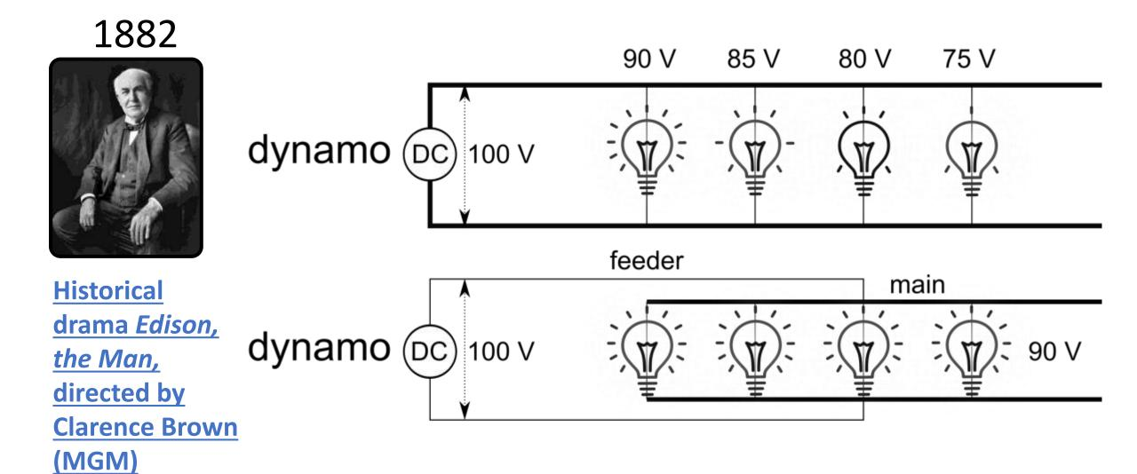
Six, 27-ton, 100-kW "Jumbo" dynamos generated the coal-fueled electric power, **Thomas Edison**'s **Pearl Street Station** transmitting 100 volts of **direct-current electricity** underground to 400 lights in a one-square-mile area of Lower Manhattan's First District (bounded by Wall Street, Nassau Street, Spruce Street, and Ferry Street).
