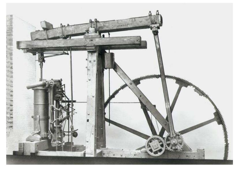
James Watt improved the condensation process by adding a separate condenser to externally cool the steam, keeping the piston cylinder as hot as possible. His engine was much smaller and used one-quarter as much coal. The modern unit of electrical power, the watt (W), or ability to "do work" or "use energy" in a prescribed time, was named in his honor.
